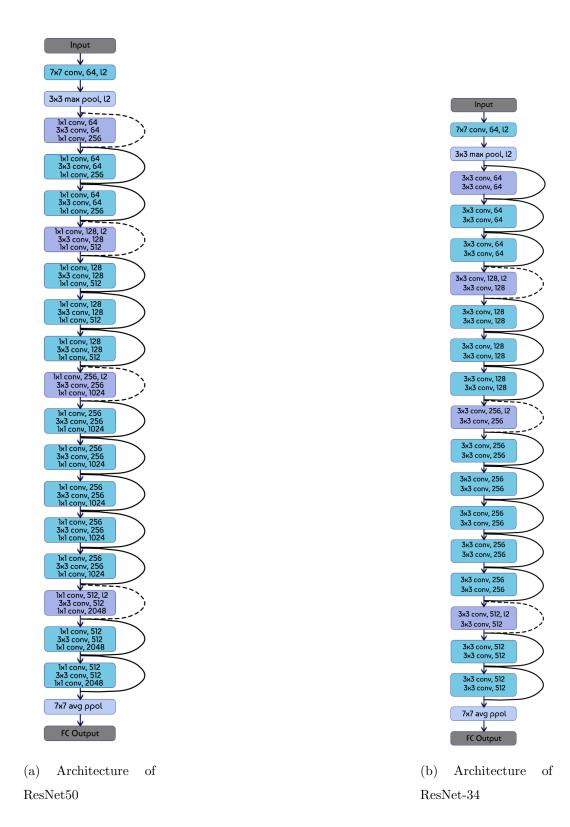
Figure 3.13: Difference Between Two Variants of ResNet Architecture.
