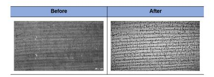
Figure 3.3: Comparison of image from dataset image before and after the implementation of CLAHE
